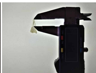
Figure 3: Conventional translucency measurement with digital vernier caliper
