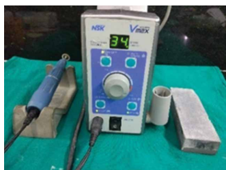
Figure 1: All the teeth were sectioned longitudinally in the buccolingual plane using Micromotor, Carborundum disc and Arkansas stone
