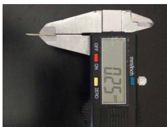
Figure 2: Confirmation of thickness of section (up to 250 \mu\text{m} ) using digital vernier caliper
