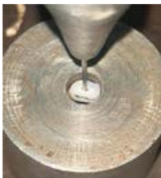
Fig.1 PBS test by Jig and Cylindrical disc
