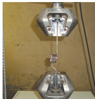
Fig1: Specimen mounted in Universal Testing Machine.
