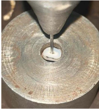
Fig.1 PBS test by Jig and Cylindrical disc
